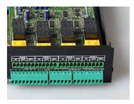
The speaker line monitoring is a plug-in board that can be optionally installed in the Spider44 / Spider04. The four zones of the line monitoring correspond to the respective audio outputs of the Spider44 / Spider04. It will short circuit, earth fault and the speaker line, but also break-down or change in level of the amplifier detected.
