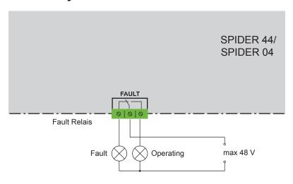
A potential-free relay contact used to display the operating status is available. In case the device is not operating or during a fault condition, the relay is released, during normal operation it is activated.
