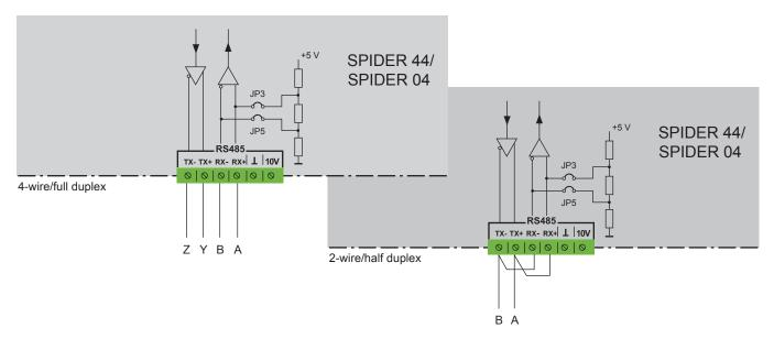
Runs in parallel to the serial RS 232 interface and is used to connect the devices mentioned before at distances of up to 500 meters. In particular, the RS 485 interface is intended for the simultaneous connection of
