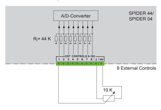
On the external control inputs a voltage of 0 to 10V is measured. These values can be used as a local gain control for the audio inputs of the device or as a control variable for the output volume of any device in the network.
