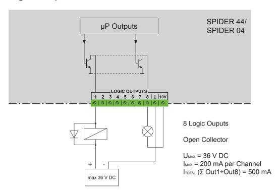
The device has 8 digital open collector transistor outputs. They are used for switching relays, lamps of lower power, etc. Typical applications are the display of faults, switching off other audio devices during an announcement and more.
