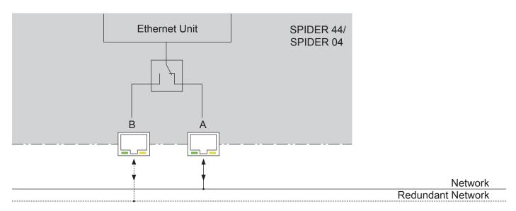
The network connection is carried out via socket A by default. If a link to second redundant network is planned, socket B is used. The LEDs on the RJ45 connector show the operating status of the network connection:
