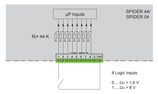
The device has 8 digital inputs, which are primarily designed for the detection of low-level operating and fault conditions. This includes the monitoring of fault signals of amplifiers, monitoring of cabinet temperature by thermostats, etc. A remote control, that is, an output follows at any point of the system the input is also possible. Each input state can be inverted for further processing by the software.
